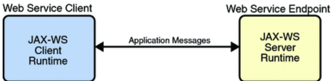
Figure 1.7. Application Message Exchange Without Reliable Messaging
